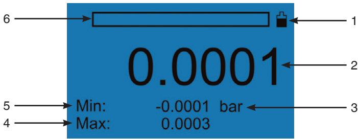
Measuring mode with MIN/MAX function
